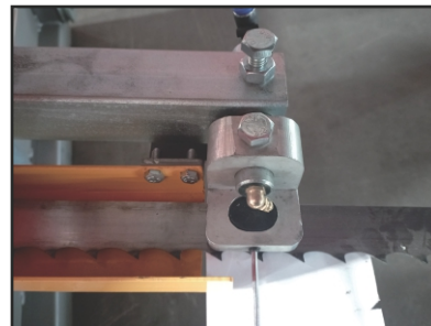
Adjust the gap below the saw blade
