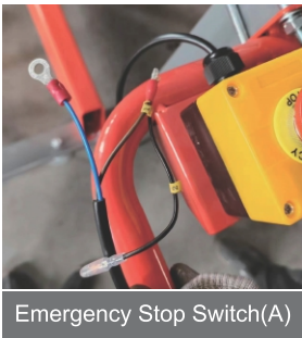
Step. 3: Find the Emergency Stop Switch(A) and the Microswitch (B)
