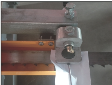
Adjusting the gap above the saw blade
